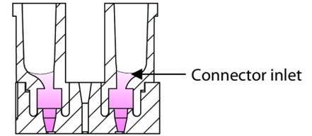
The medium levels should be the same as or slightly above the level of connector inlet
