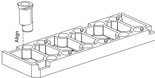
3. Press connectors down into AIM chips to make sure the contact areas between the connectors and the AIM chips are flush.
